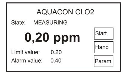
The automatic analysis cycle can be interrupted at any stage by touching the button "Hand" or the button "Param" on the touchscreen (see 3.5). After the finish of the analysis, the new measured value will be displayed on the touchscreen and the analyzer state is changed to "STANDBY" (see 4.2).
